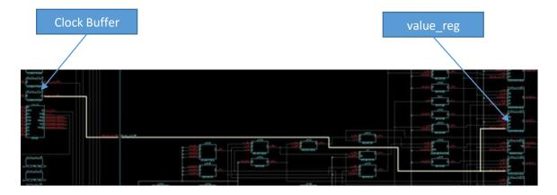
To watch the delay in the simulation output, we can add the Z and CK pins to the waveform. Be careful, we want to see the signal at the Z and CK pins, not the wire itself. To do so, you have to click on cell's PIN not the wire, like this:
