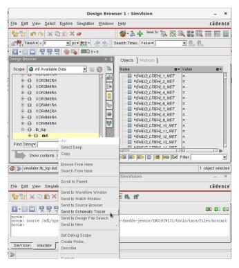
To do so, open the schematic tracer on the "dut":
