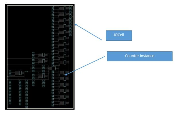
Now you can zoom around the counter instance, and double click it to open its internal schematic.
